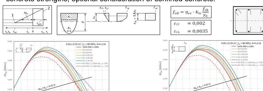
Note consistency between capacity based on parabola-rectangle and based on stress block
