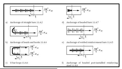
$$l_{\rm bd} = k_{\rm lb} \cdot k_{\rm cp} \cdot \phi \cdot \left(\frac{\sigma_{\rm sd}}{435}\right)^{n_{\sigma}} \cdot \left(\frac{25}{f_{\rm ck}}\right)^{\frac{1}{2}} \cdot \left(\frac{\phi}{20}\right)^{\frac{1}{3}} \cdot \left(\frac{1.5\phi}{c_{\rm d}}\right)^{\frac{1}{2}} \ge 10\phi \tag{11.3}$$
