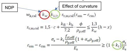
Simplified control of cracking moved to Informative Annex
